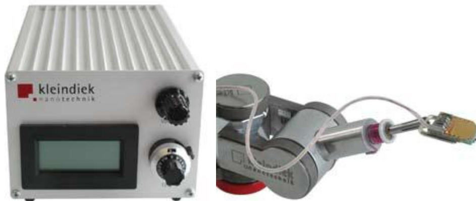
Figure 5: FMS controller and force measurement tip in holder mounted on a micromanipulator [8]
