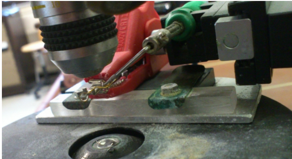
Figure 3.9: The setup for the micropolishing. The gold wire with the H_2SO_4 film can be seen; when the picture was taken there was no contact between the film and the microwire.
