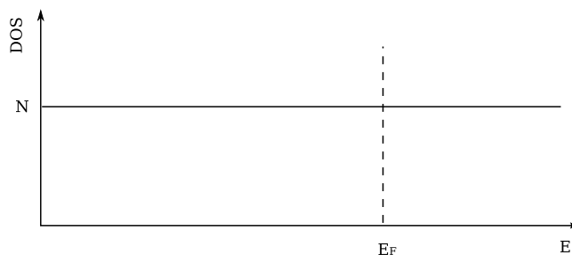
Figure 6.3: Constant density of (trap) states as used by Mott for his transport model. E_F denotes the Fermi energy.
