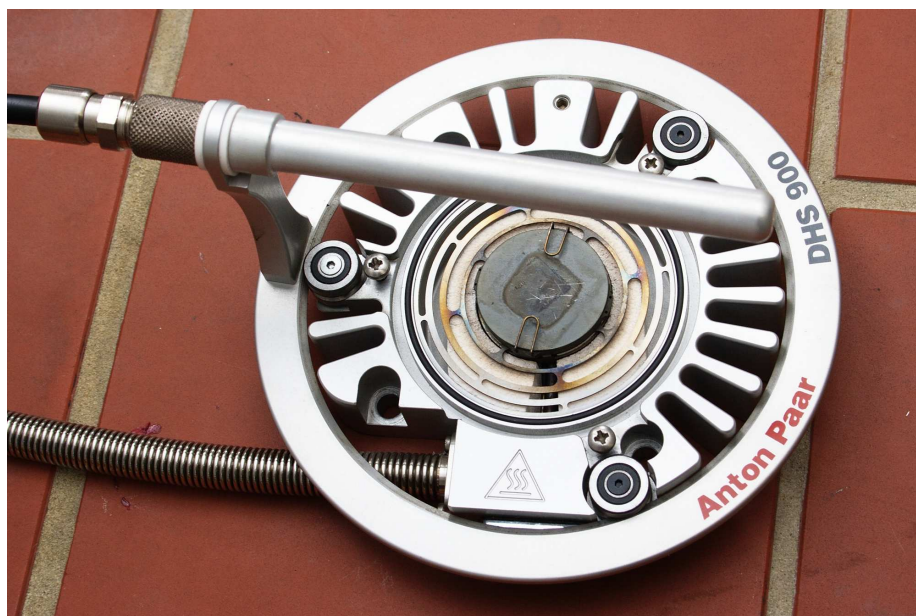
Figure 10.9: DHS 900 heat stage from Anton Paar company used for heating experiments in the glovebox.
