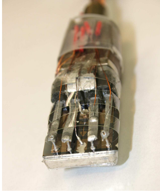
Figure 10.5: Photo of the original sampleholder with installed sample.
