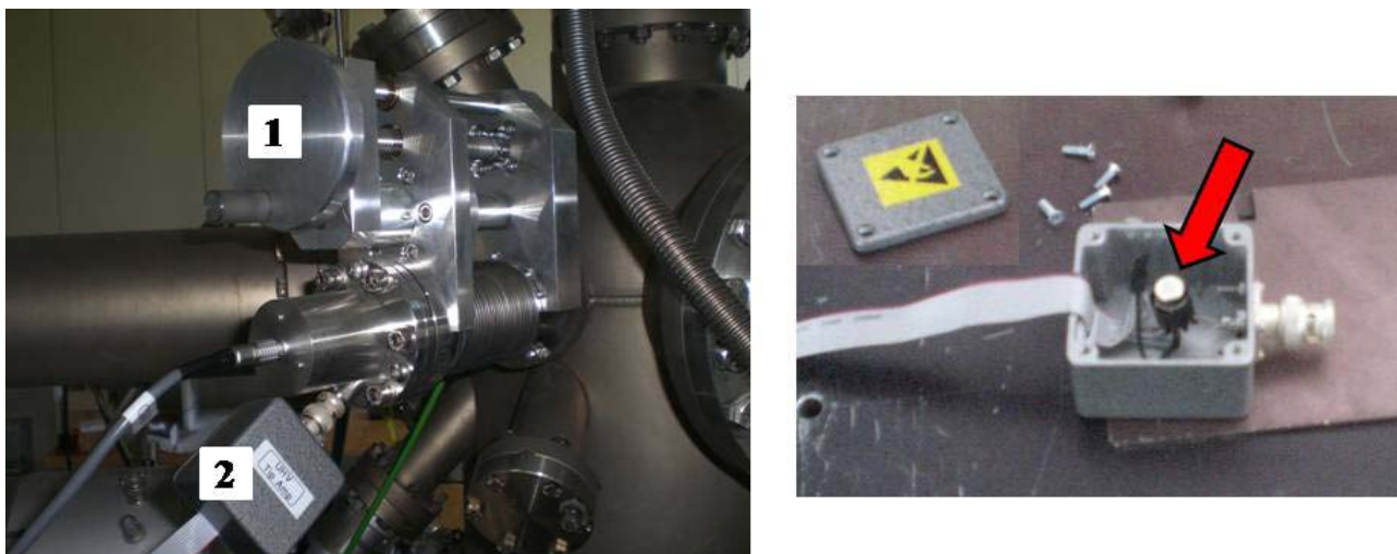
Fig. 10.16: Left: Photograph of the UHV Kelvin probe. 1: Positioning wheel to approach or withdraw the tip, 2: UHV tip amplifier. Right: Detail and interior view of the UHV tip amplifier. The red arrow points to the electronic component that must be replaced if the signal remains constant at 13\text{ V} .
