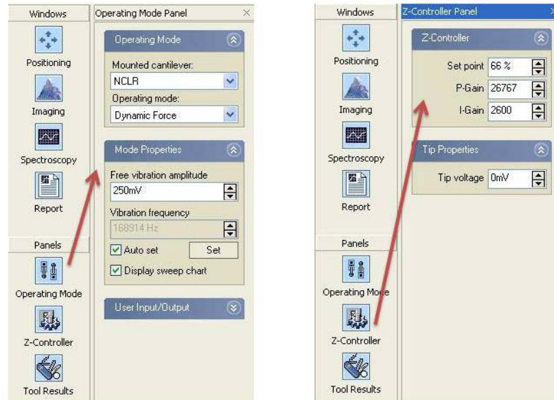
Fig. 10.6: Left: Operating mode panel ; The mounted cantilever is a non-contact cantilever ( NCLR ) and the AFM is run in the dynamic force mode. Here the free vibration amplitude can be optimized. Right: Z-controller panel . Here the set point and the loop gains can be optimized. The tip voltage is not used in this mode.
