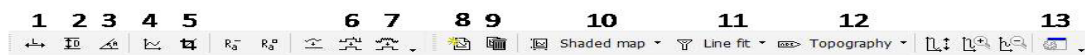
Fig. 10.7: Image processing bar; 1: Measure length; 2: Measure distance; 3: Measure Angle; 4: Create cross-section; 5: Cut out area; 6: Glitch filter; 7: Noise filter; 8: Create new chart; 9: Delete chart; 10: Select chart type; 11: Select data filter; 12: Select signal; 13: Show chart properties dialog;
