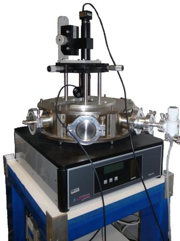
Figure 3.2.: Photograph of the assembled light microscope station.
