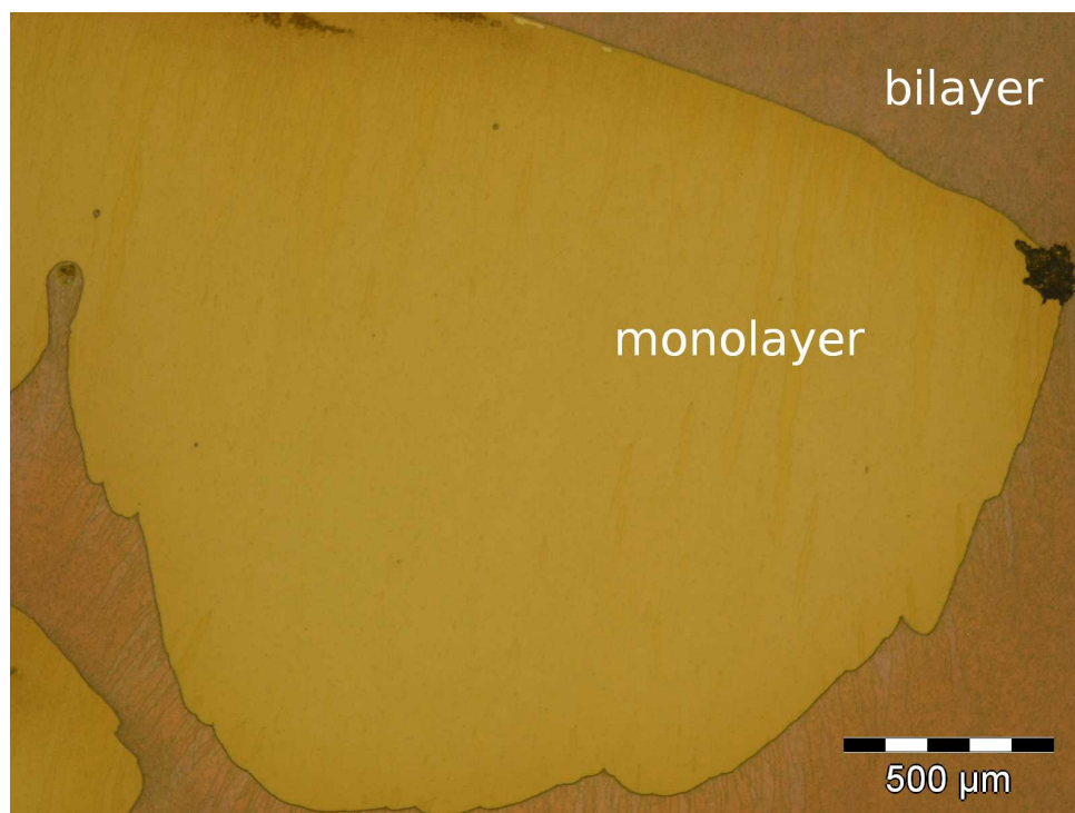
Figure 5.10: Optical micrograph of a close-packed monolayer region PS sphere diameter: d = 500 nm
